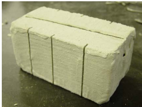
Figure 3.19. Break locations for round 2 testing and a sample waiting to be broken for testing.
