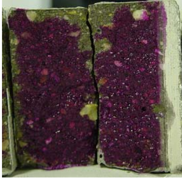
Figure 2.1. Photo of concrete surface sprayed with phenolphthalein. Magenta color indicates pH greater than 9, which colorless area indicates pH less than 9.
