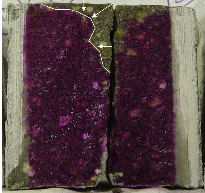
Figure 3.22. Round 2 sample showing inward curve carbonation front. Arrows indicate the direction of the gas penetration and subsequent carbonation front progression.
