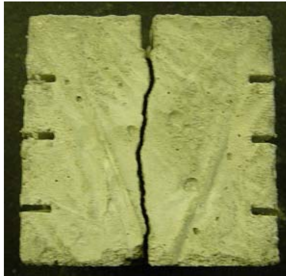
Figure 3.14. Schematic showing break locations used during round 1 for phenolphthalein testing and a sample waiting to be broken for testing.
