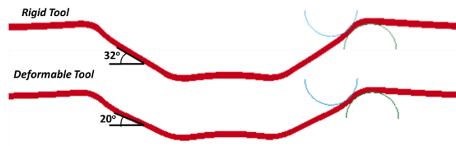
Figure 3.25 Cross-section comparison between rigid tool and deformable tool simulation models
