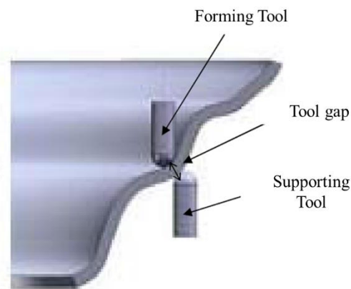
Figure 2.3 Schematic showing the tool gap in DSIF (Malhotra et al., 2011)
