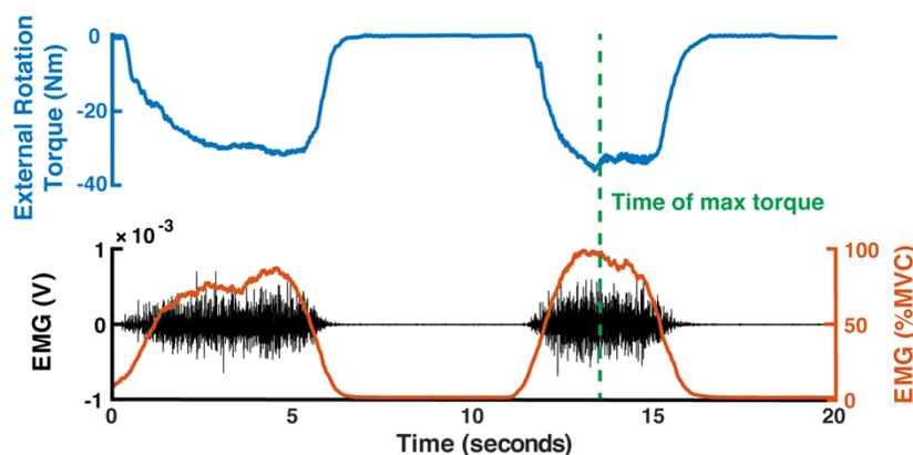
**Figure 2.3. Raw and filtered EMG and torque**
