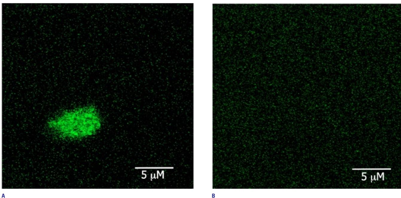
**Figure 11.** Sonication after NHS linker reaction removed any extreme DNA clumping. (A) A fully functionalized DNA surface was imaged without sonication in toluene after the NHS linker reaction. This resulted in large clumps of fluorescently tagged DNA. (B) A fully functionalized DNA surface was imaged with sonication in toluene after the NHS linker reaction, resulting in less clumping on the surface.
