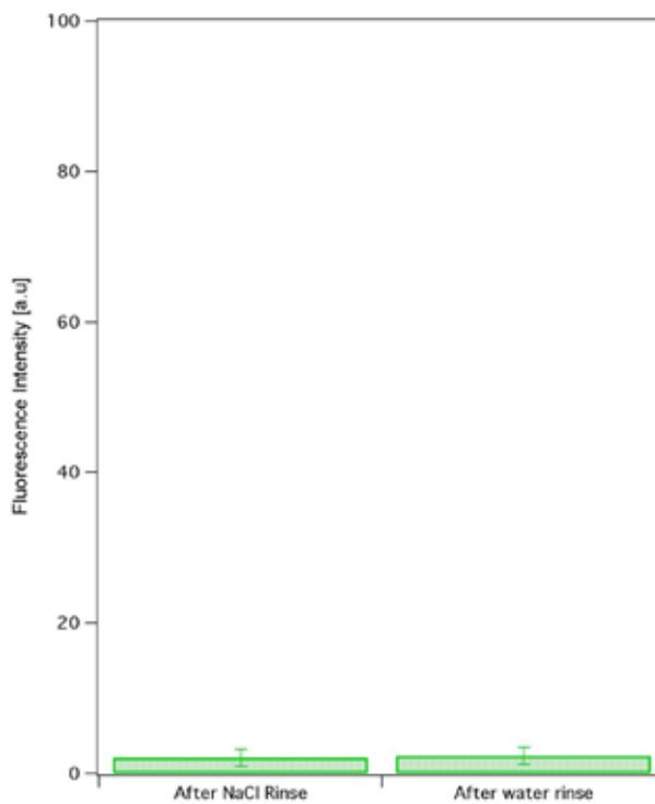
**Figure 10.** Binding study of the complementary strand to the NHS linker surfaces. The NHS linker surface was exposed to a solution of the tagged  $A_{25}$  to test if the complementary strand nonspecifically bound to the linker. No fluorescence was observed in the image after both a 0.25 M NaCl rinse and a water rinse.
