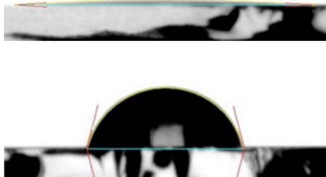
**Figure 4.** Contact-angle measurements of a silica surface and a NHS-functionalized silica surface. Two images taken of a water droplet of the same sessile volume ( $\sim 2 \mu\text{L}$ ) on two different surfaces using a contact-angle goniometer. The first surface is the hydrophilic glass slide. The contact angle measured for this surface was  $3.9^\circ$ . The second surface, the NHS linker surface, exhibited a high contact angle of  $75^\circ$ .
