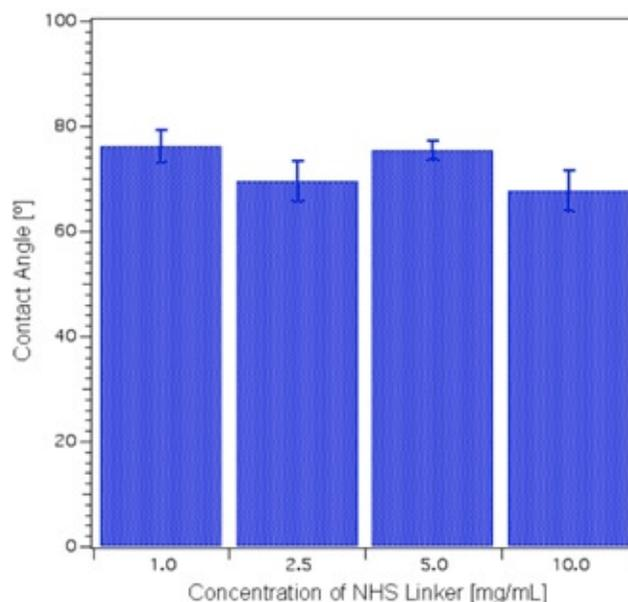
**Figure 6.** NHS linker concentration minimization study. Contact-angle measurements were taken after the NHS linker reaction at various NHS linker concentrations in toluene.
