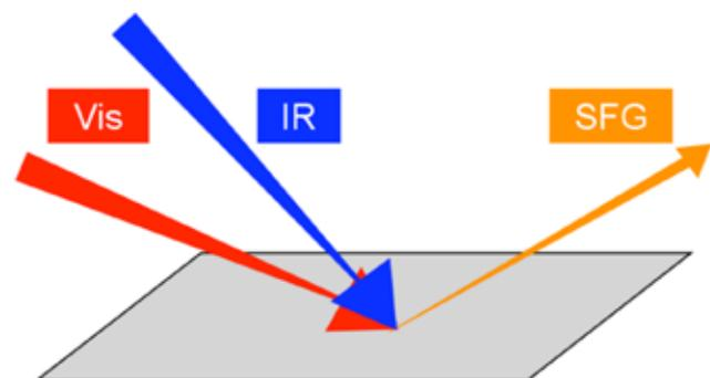
**Figure 2.** Sum frequency generation description. SFG is a nonlinear optical technique used to characterize DNA. Visible and IR beams are directed at the surface-bound DNA to produce a beam at the sum of their frequencies that contains vibrational information about the identity and orientation of the molecules at the surface.
