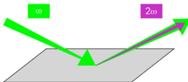
**Figure 1.** Second harmonic generation description. SHG is a nonlinear optical technique used to characterize surface-bound DNA. Photons of a certain wavelength are directed at a nonlinear material, such as a silica/water interface, at which point their frequencies are doubled.
