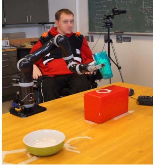
Figure 7.5. An SCI user controlling the robot with the BMI during the experimental task.
