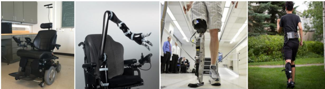
Figure 1.1. Examples of assistive human-robot systems. Powered wheelchair (Northwestern University), JACO robotic arm (Kinova, Canada), Prosthetic leg (Shirley Ryan AbilityLab, USA), Exosuit (Harvard University).
