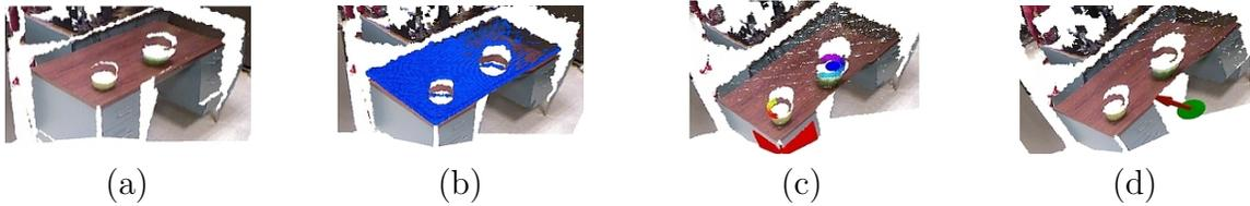
Figure 5.4. Example of the object anchoring approach. (a) Point Cloud of the scene with image overlay. (b) Candidate surface extraction (blue region). (c) Object Clusters (rainbow-colored circles), Hough Circle Detection (blue marker) and 3D box (red box). (d) Identified docking location (green marker) and docking pose (red arrow).
