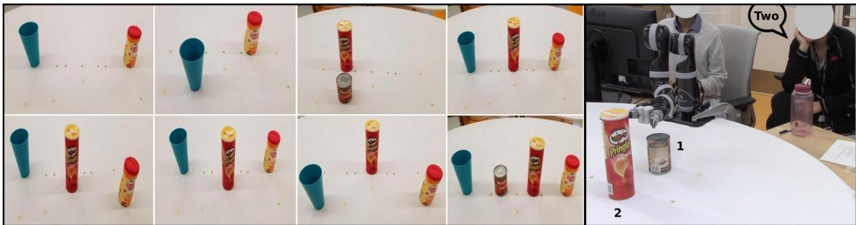
Figure 6.3. *Left*: Goal scenarios of varied complexity used in human inference study. *Right*: Example setup shows the robot executing a trajectory to reach a goal. The subject predicts the intended goal during robot motion.
