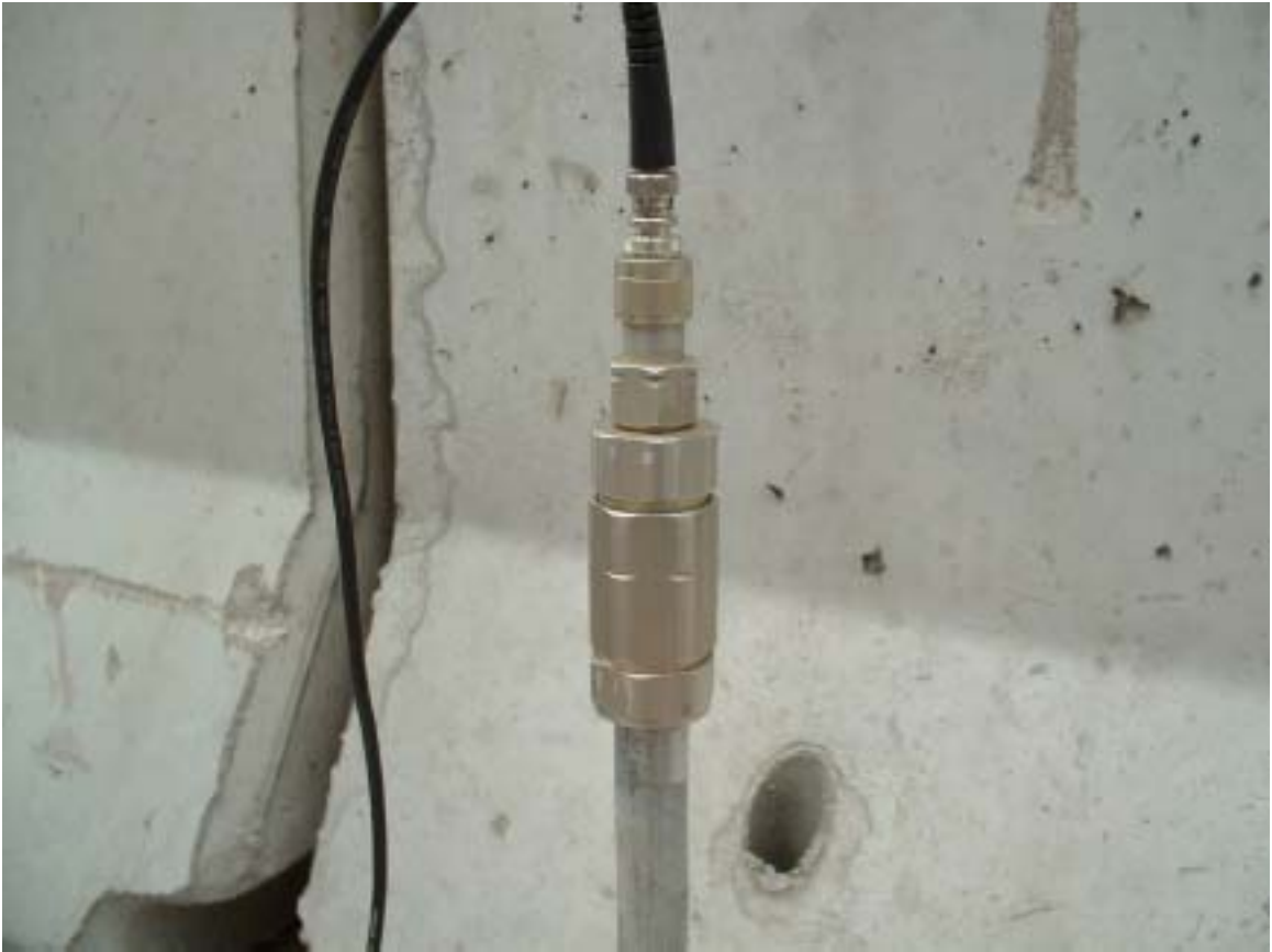
TDR cable equipped with a GRS F type connector and a lead cable for interrogation
