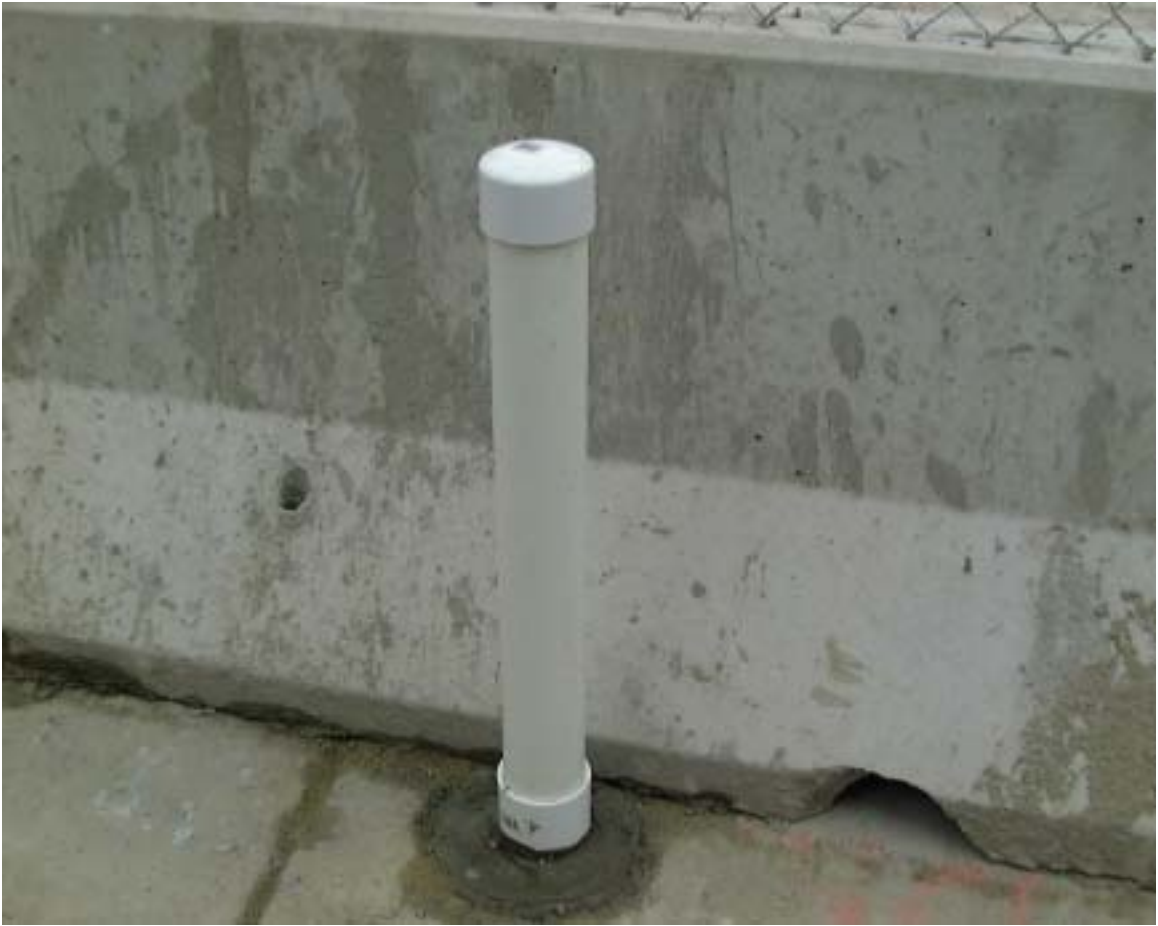
Sealed PVC casing protecting a TDR connector
