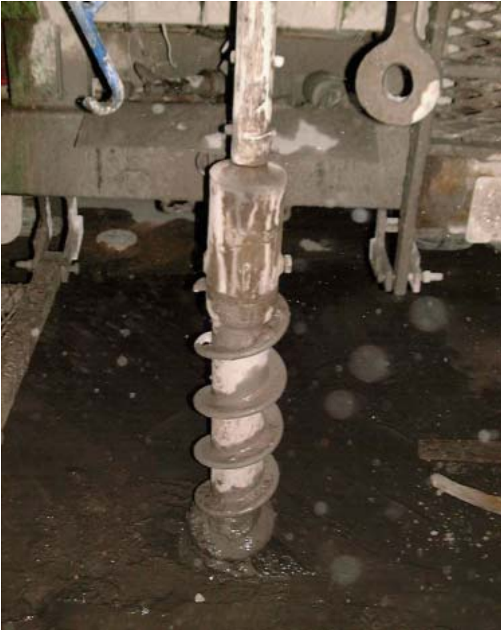
Close up on a hollow stem auger, drilling in soft Chicago clays
