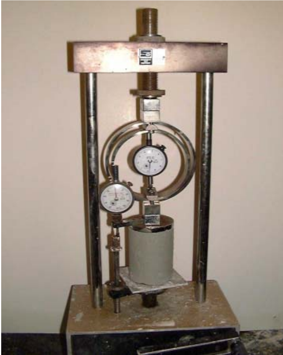
Figure 6-8: Soiltest unconfined compression machine used to test grout mix samples.
