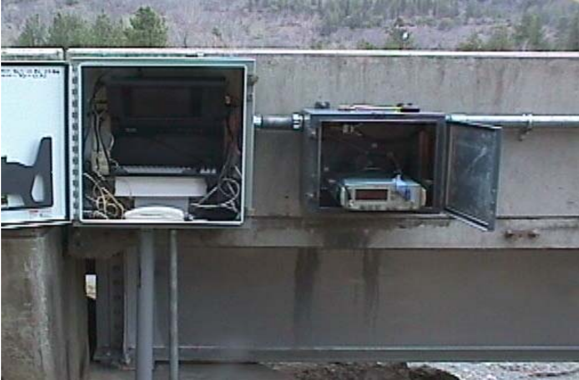
Figure 2-17: View of the first DAS installed at Horse Creek, CA, with the PC on the left and the Textronix cable tester 1502 on the right.
