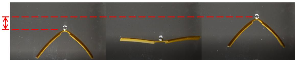
Figure 5.5: Hydrogel swimmer demonstrating underwater locomotion in the lab. The three snapshots are taken in chronological order from left to right.
