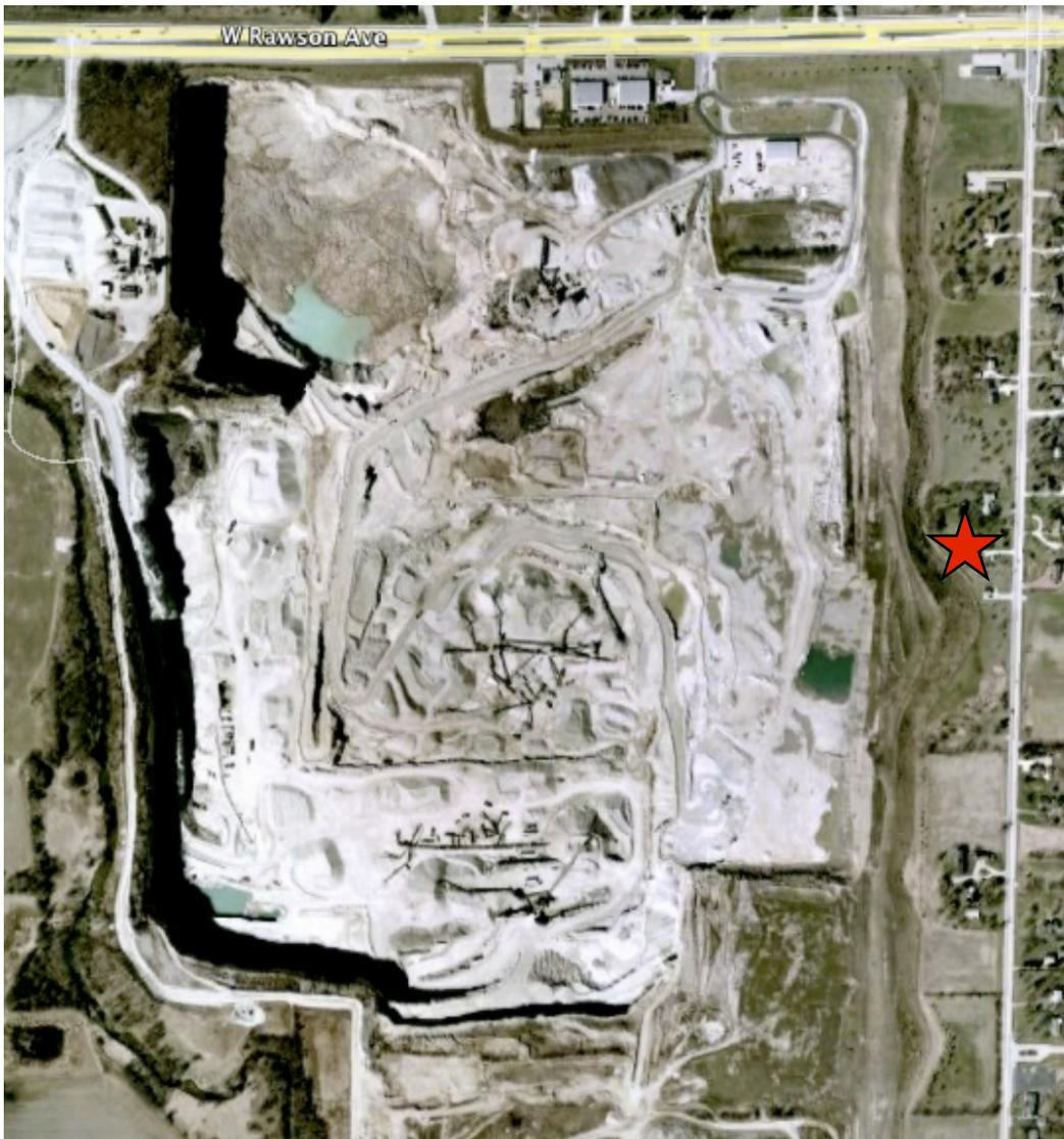
**Figure 2** - The red star indicates the location of subject house in Franklin, Wisconsin just east of the Vulcan Quarry. The test house is representative of a home closest to the quarry with blasts between 1500 and 2000 feet away.
