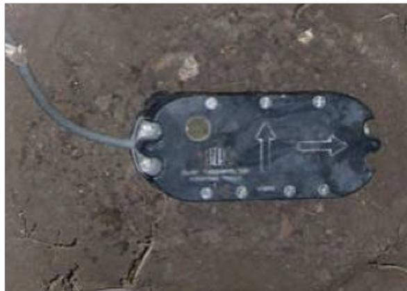
**Figure 5** - Triaxial Ground Motion Sensor
