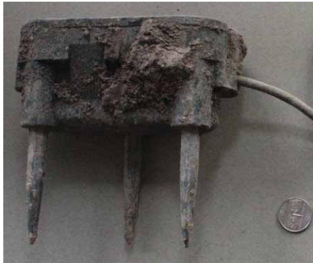
**Figure 2.6:** Photograph of a triaxial geophone with quarter for scale
