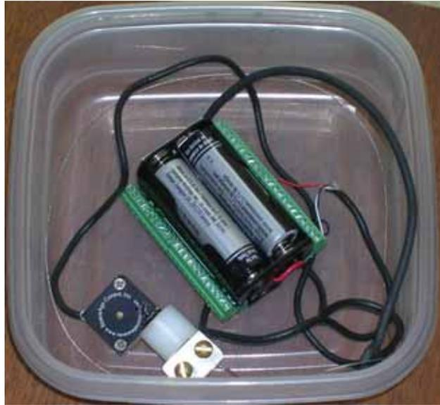
**Figure 3.14:** A typical mote in a plastic container
