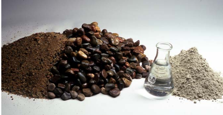
Figure 2-1: The basic ingredients of concrete. From left to right: fine aggregate (sand), coarse aggregate (gravel or rocks), water, and cement. (Image courtesy of the Portland Cement Association). MK5-019
