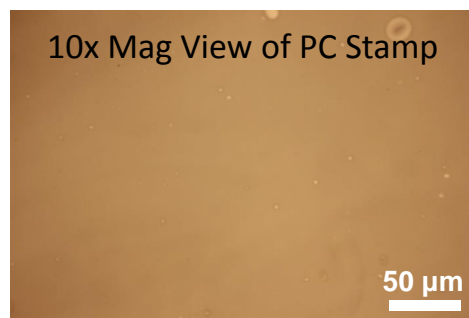
Figure A.13. (a.) Cut down stamp on glass slide, anchored with gel. Note the transparency and lack of trapped bubbles. (b.) Stamp under the microscope. (c.) Stamp as seen by the microscope, note the uniform, transparent nature of it with no visible chunks of PC.
