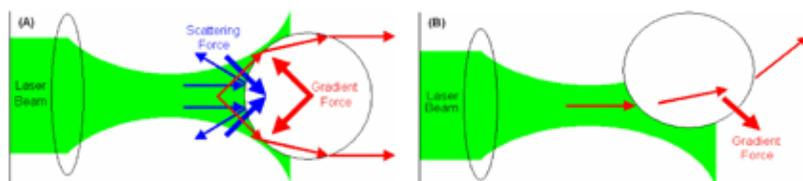
**Figure 1:** Diagram illustrating the gradient and scattering forces on a particle caused by the change in momentum of the light. (A) illustrates a particle in equilibrium. (B) illustrates the gradient force pulling the particle towards the center of the beam.
