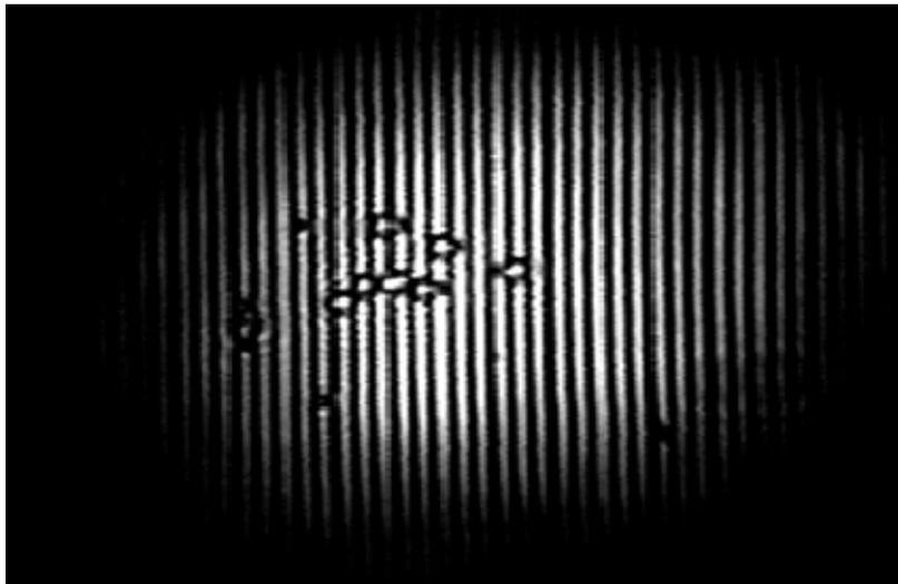
Figure 5: Image of the optical standing wave. Particles can be seen “trapped” on the white lines, which are the standing-wave intensity maxima.
