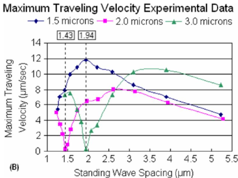
Figure 3: Graphical representation of the (A) theoretical and (B) experimental values for the maximum displacement velocity for differently sized particles. The theoretical curves show the absolute value obtained from the Rayleigh scattering theory. The dashed lines in (B) represent standing-wave spacings corresponding to a vanishing optical force on the particle (where it always slips). These standing-wave spacings are the basis of the optical sorting process.
