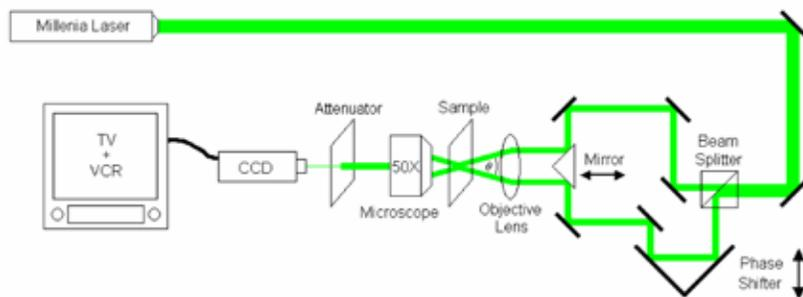
**Figure 2:** Schematic of the interferometry setup. The phase-shifting mirror is mounted on a piezoelectric displacer that is in turn mounted on an optical translator.
