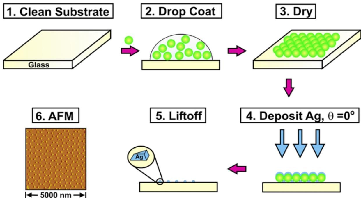
**Figure 1.** Fabrication of Ag nanoparticles via nanosphere lithography (NSL). (1) Glass substrate is cleaned. (2) Polystyrene nanosphere solution is drop-coated on to the glass. (3) Nanosphere solution is dried in ambient conditions. (4) Nanospheres form a hexagonally close-packed array. (5) Deposition of Ag onto nanospheres. (6) Removal of nanospheres by sonication. (7) AFM image of triangular Ag nanoparticles.
