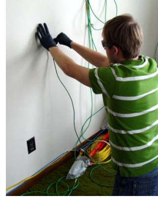
Figure 9: Applying Pressure while Epoxying LVDT
