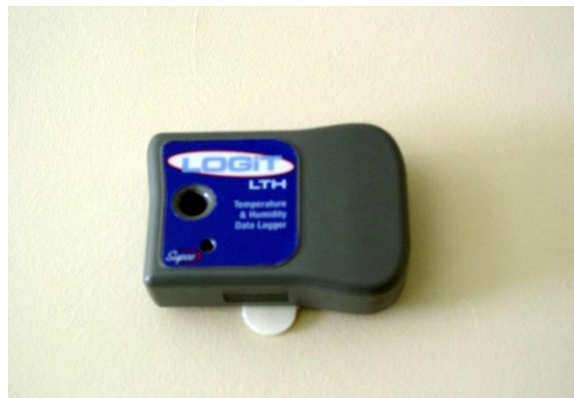
Figure 16: SUPCO Temperature and Humidity Gauge
