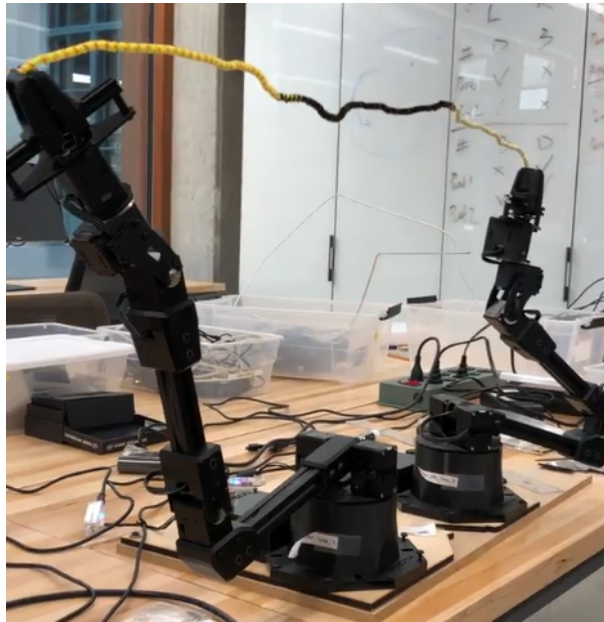
Figure 5.4. Two WidowX 200 robots grip the ends of a pipe cleaner and reconfigure it in physical experiments.
