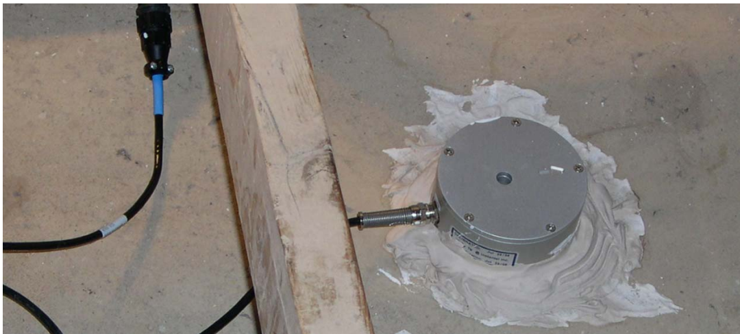
Figure 5.2 Installation of the geophone in the downstairs of the test house.
