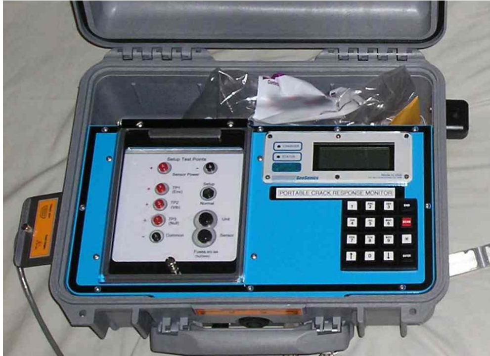
Figure 2.6 External key pad for on-site programming of the system X crack monitor.
