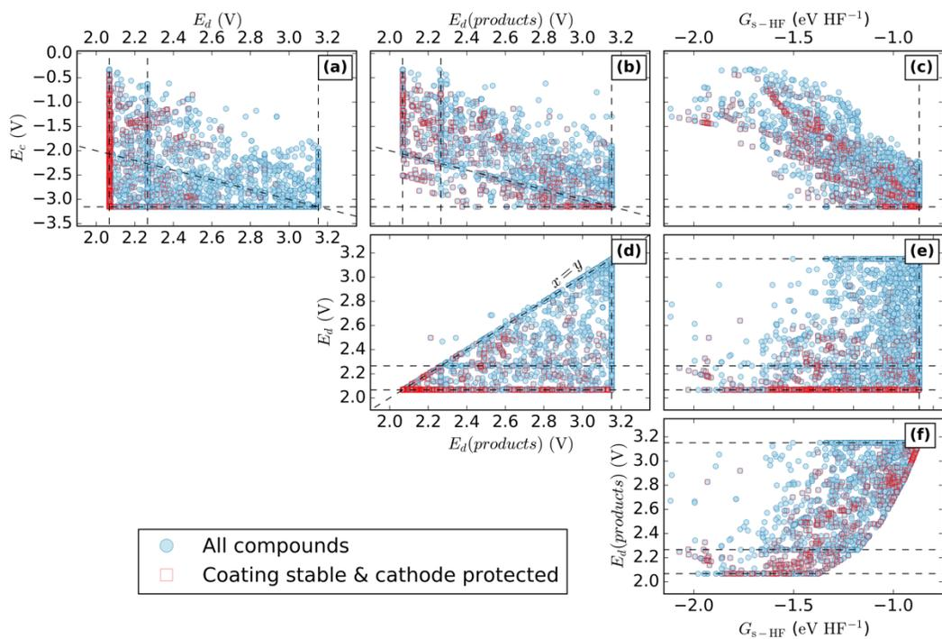
Supplementary Fig. 1. Coating attribute matrix in presence of LiCoO<sub>2</sub>. Each subplot from (a) to (f) in the matrix plot compares pairs of attributes when LiCoO<sub>2</sub> is included in the chemical space.
