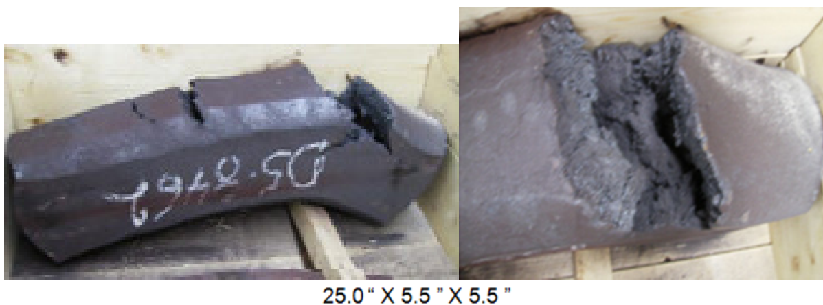
Figure 6.1.4: As-received ingot of SA-120 showing incipient melting and wide-cracks
