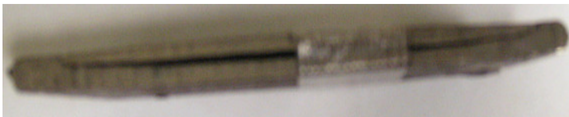
Figure 6.1.3: Cut-off piece from the as-received plates of BA120 with thickness of ¼ in showing the delamination of the plates being held together by tape
