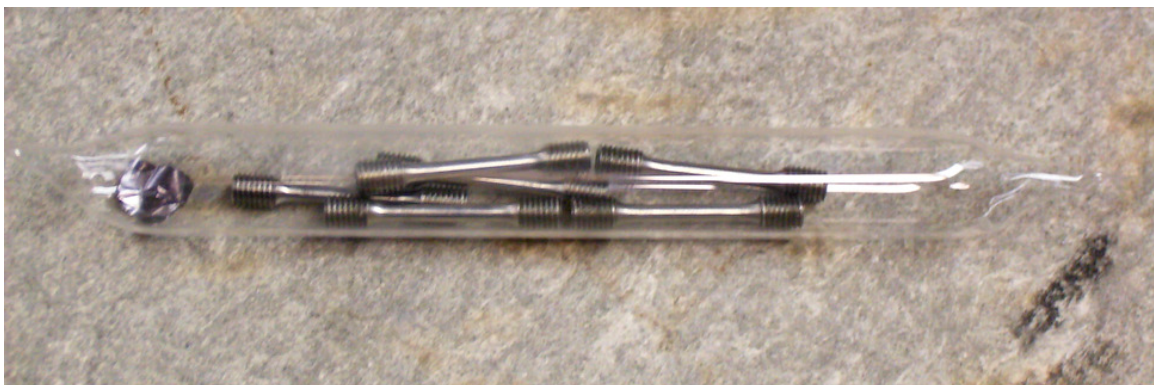
Fig 3.3.1: Tensile bars vacuum encapsulated and sealed in a glass tube prior to aging. A small piece of tantalum foil can be seen at the left corner to absorb the trace oxygen in the system
