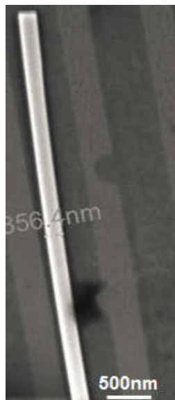
Figure 6.1.5 The SEM image of a single gold nanowire array grown inside a channel. The width of nanowire is about 350nm, the channel width is about 800nm
