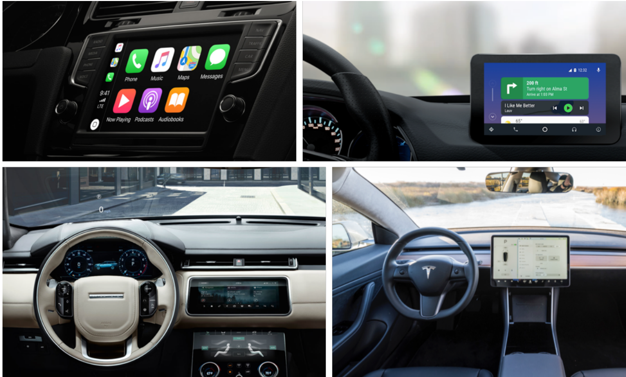
Figure 2.2: (clockwise from top-left) Apple CarPlay [71], Android Auto [70], Tesla Model 3 [74], and Range Rover Velar [75]. CarPlay and Android Auto mirror content from a mobile phone onto a car's inbuilt infotainment system. The Model 3 & the Velar have large touchscreens that are used for changing vehicle parameters and serve all multimedia needs.
