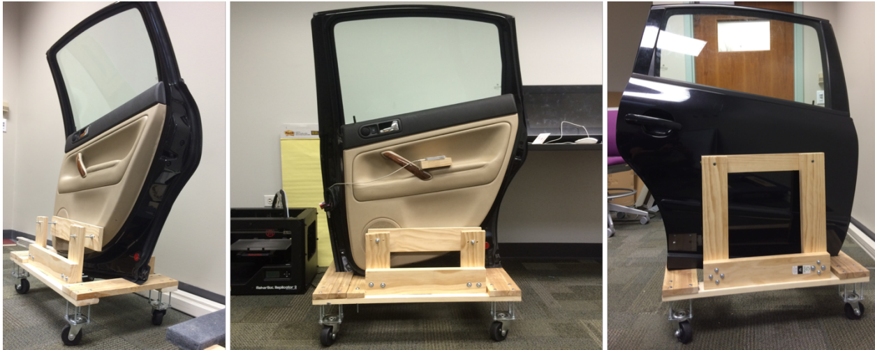
Figure 3.1: A passenger door from a 2005 VW Passat mounted on a wooden frame. The assembly was designed to be easily wheeled around; and had height-adjustable wheels (this was also used to level the platform).
