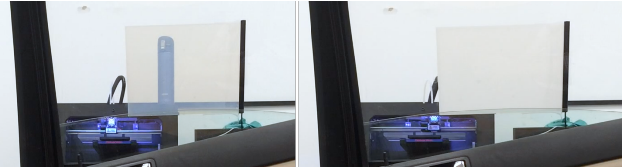
Figure 3.2: Switchable film that can be made transparent or opaque by passing electricity through it. This particular film was purchased from Smart-Tint [51].
