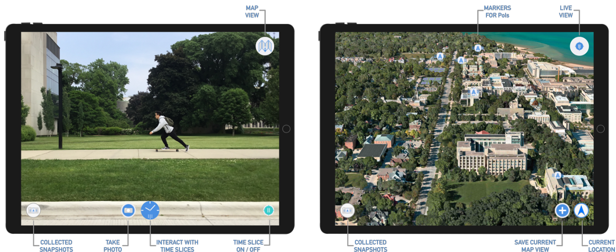
Figure 5.4: Two distinct views, Live View (left), and Map View (right). Live View allows Time Slicing, taking a snapshot, and reviewing saved snapshots. Map View allows one to look at PoIs, and explore by using pan and world-tilt gestures, and also review saved snaps
