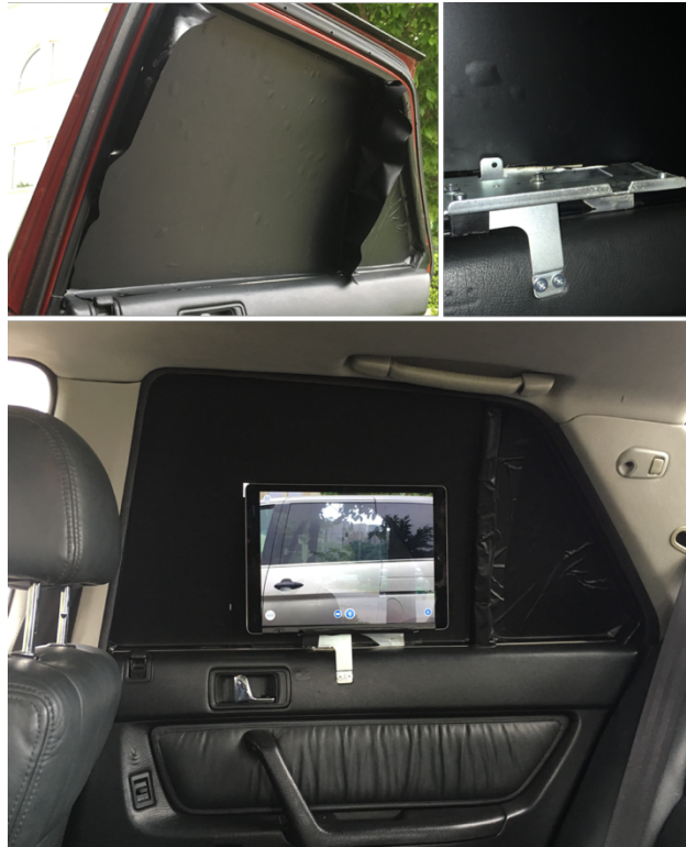
Figure 5.2: Blacked out rear window (top-left), a platform with a lip that the iPad rested against (top-right), and the iPad's camera aligned with a hole in the blacked out window (bottom).
