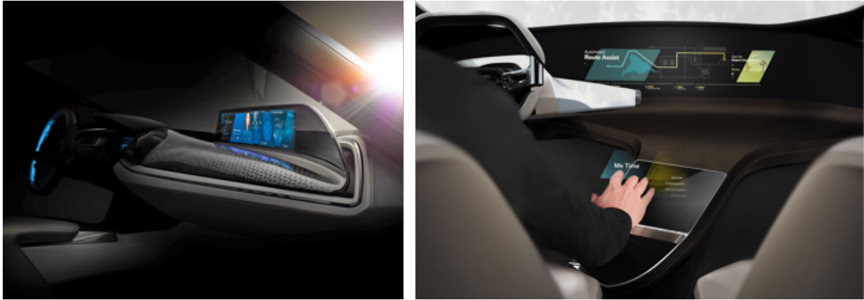
Figure 2.5: BMW's AirTouch [68] and HoloActive Touch [47] concepts are designed to work with in-air gestural input from drivers and front passengers.
