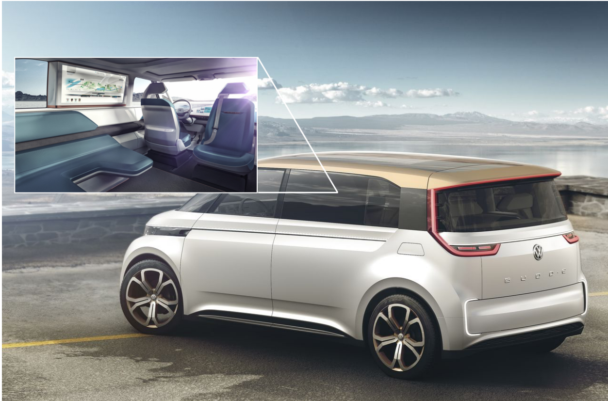
Figure 2.4: The Volkswagen Budd-E concept car has a large display on a passenger side window that is used for productivity tasks and video conferencing during travel.
