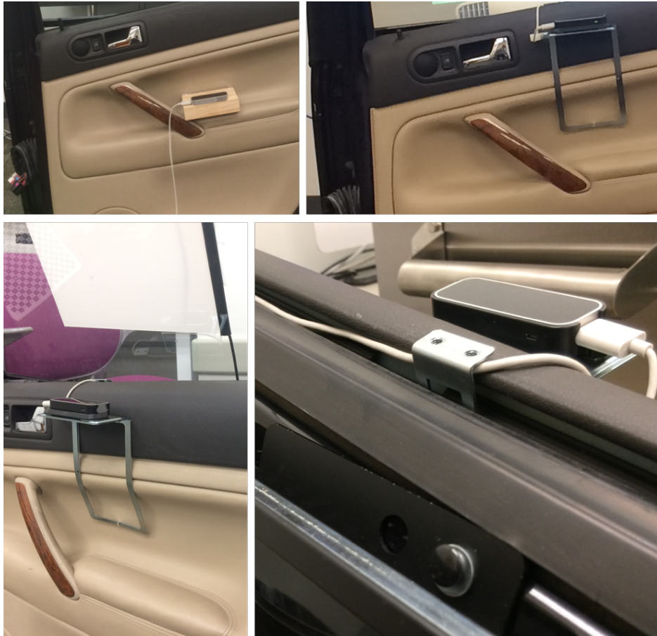
Figure 3.6: The Leap Motion controller [48] was mounted on the arm rest, but that was too low. It was moved closer to the window sill for more accurate tracking.
