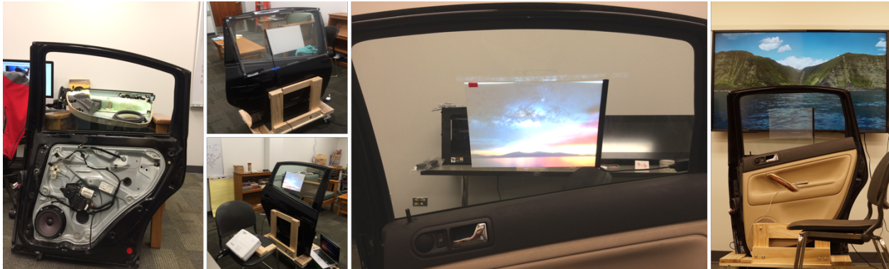
Figure 3.3: (From left to right) I removed the built-in window; attached a 0.1” thick acrylic sheet to the infra-red multi-touch frame to the window and stuck the switchable film onto this sheet; rear-projection on the switchable film while it is opaque; 65” TV screen behind the door to show the external world (note, the height of the TV relative to the door was adjusted later).
