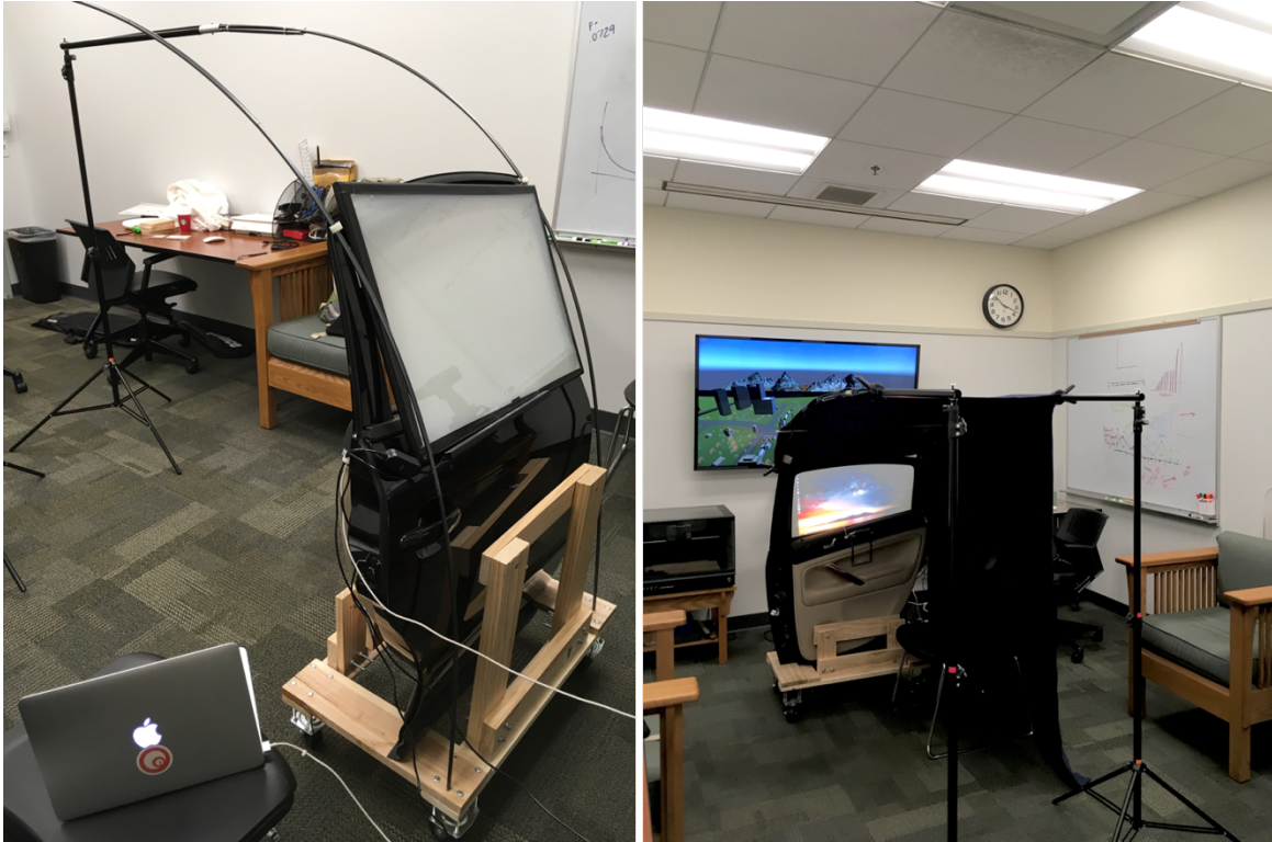
Figure 4.2: Tent poles connected to studio tripods (left) formed a structure that was used to drape a cloth over the car door to make a canopy (right). The window display was significantly larger than the prior iteration.
