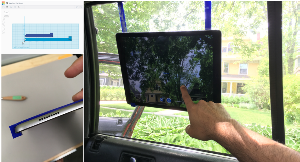
Figure 5.1: Initial design of the mount was an elongated s-shaped hook that supported the iPad on one end and hooked onto the top of the window on the other. Velcro strips on the back of the iPad kept it flush with the window.
