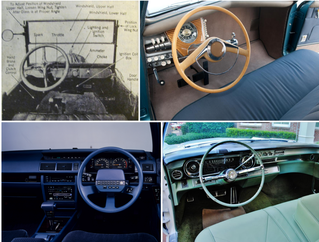
Figure 2.1 (clockwise from top-left): 1923 Ford Model T [64,66] with an ammeter as the only dial on the dashboard; the 1948 Tucker Torpedo [65] with a lot more dials and switches; the 1965 Cadillac Deville [63] with an A/C and radio on the dashboard; the 1988 Nissan Heritage [33] with a car phone and digital displays driven by an onboard computer .
