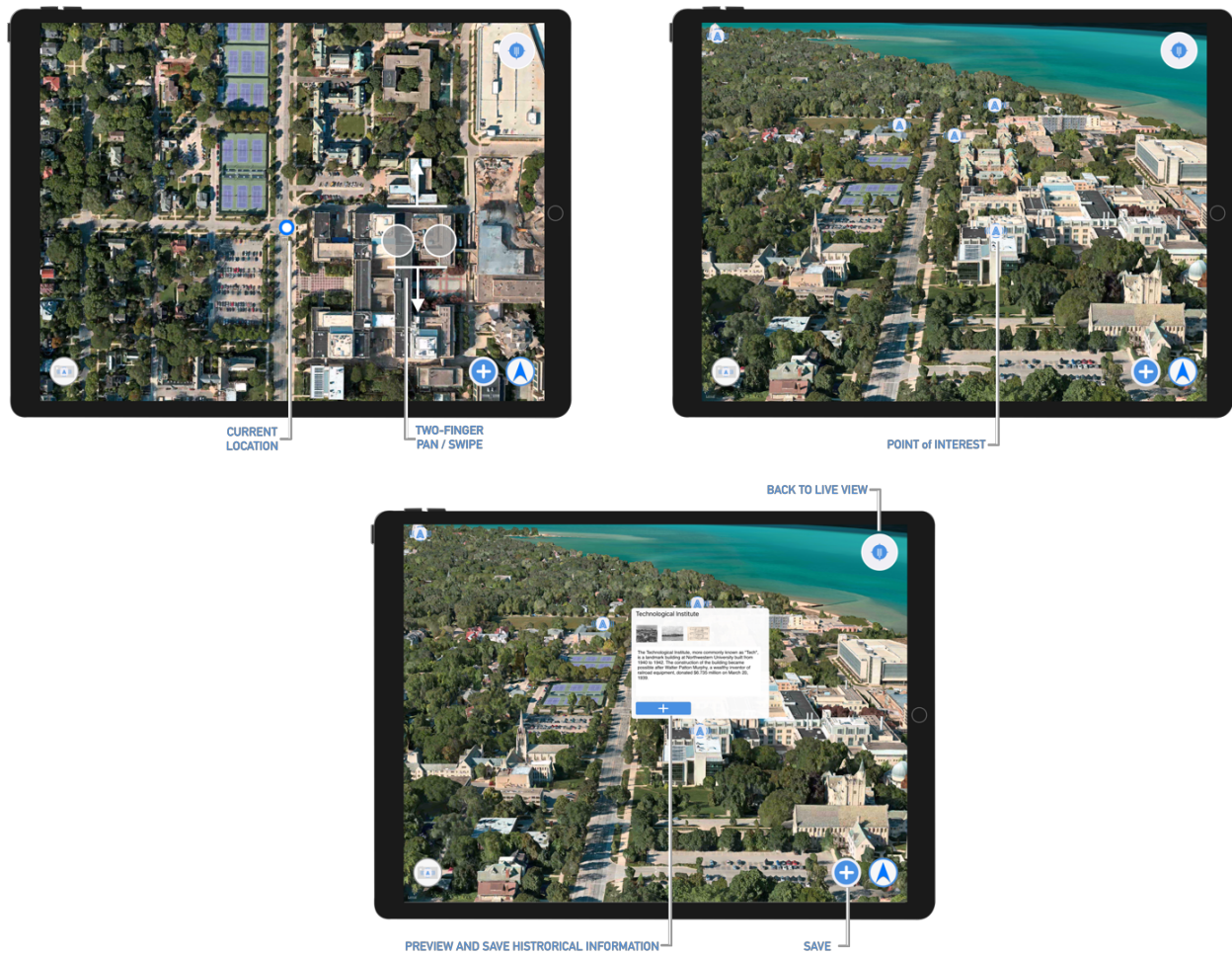
Figure 5.6: Map View showed a satellite view initially centered on the current location. A two-fingered pan/swipe (same as World Tilt in the lab) showed the 3D representation. PoI's were annotated with "A" markers. A user could save the map view or an image of the PoI.
