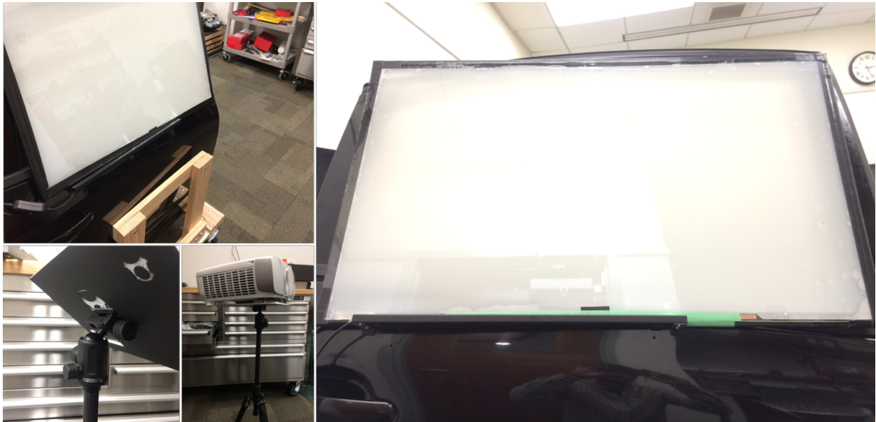
Figure 4.1: Acrylic layer replaced with glass; it needed a sturdier aluminium mount (top-left, right), the switchable film now spanned the entire window (right), and the projector was mounted on a tripod by repurposing a plastic board.
