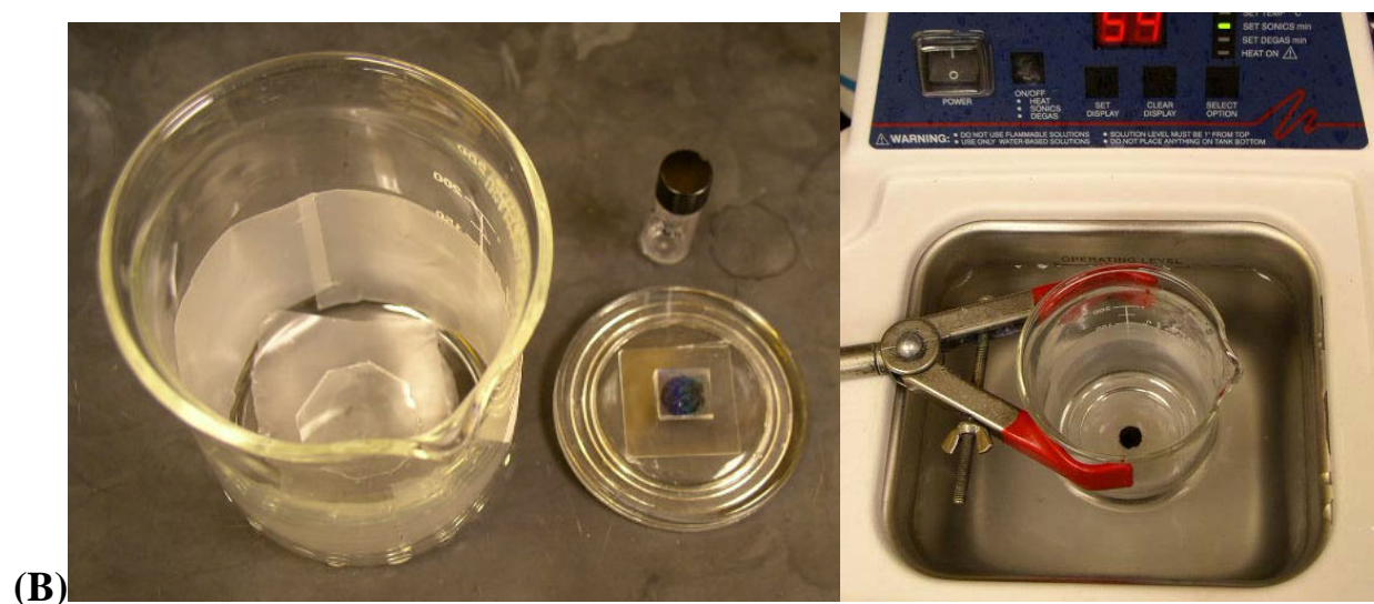
Figure 4.1. (A) Schematic briefly detailing the two patterning methods employed and (B) photographs of the setup used for sonication-assisted solution embossing.
