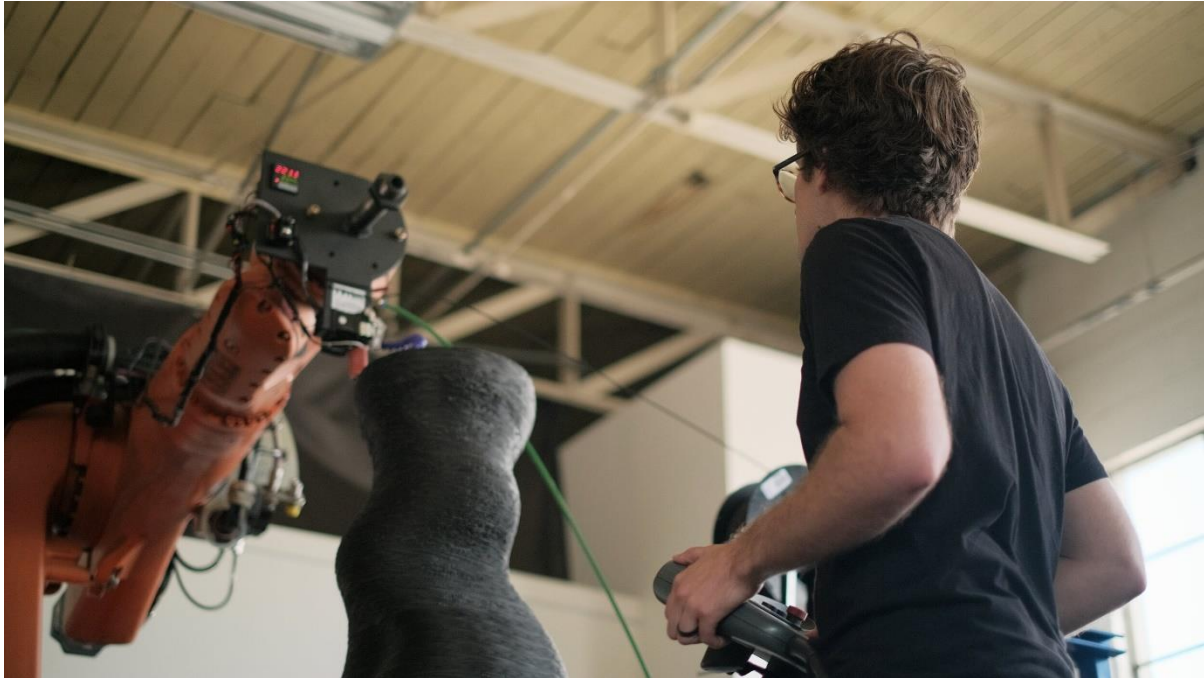
Figure 30 - Photograph of Cody using a Kuka KR-16F industrial robotic arm while in residency at Ballard International. The printing of the Turbulence vessel can be seen (Norman, 2020c; Norman, 2021a).
