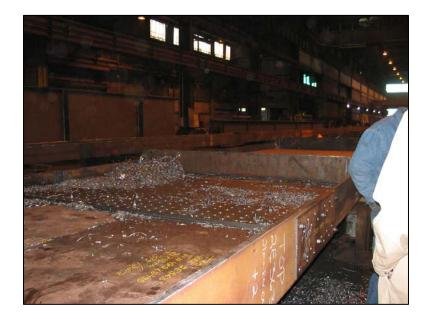
Figure 3. Holes are drilled in girders
