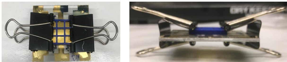
Figure 2.9: Photographs of 3D printed 3x3 wells sealed with PPL array. Clamps were used to compress the wells into the elastomeric PDMS to for a seal between each well.
