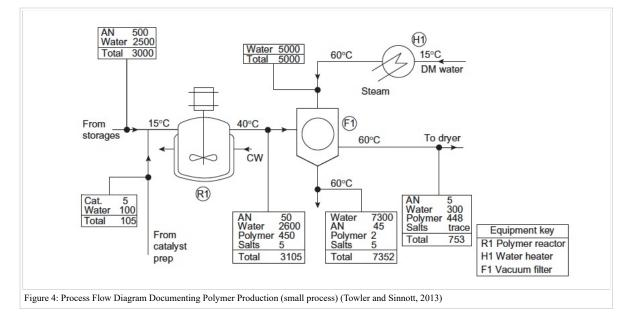
A new process flow diagram was created in order to avoid the clutter of this first process flow diagram. Note that the streams that are labeled are just the numbers, with their stream information detailed in a separate table (Table 7).
