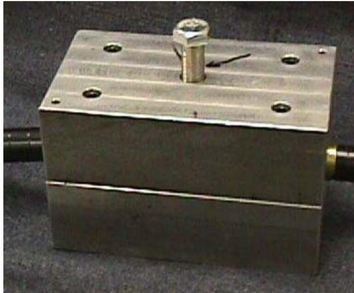
**Figure 3-3. Photograph of the assembled apparatus. The bolt is replaced by a piston for measurement of force-displacement response (Cole, 1999).**
