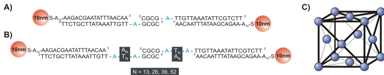
Scheme 4.1. Materials Sequence and Design. A) Illustration of the three-dimensional arrangement of particles forming a face-centered cubic lattice showing the effect of increasing linker length on lattice parameters, B) sequences of oligonucleotides used to form the various N = X linkers ranging from 13 duplex spacers up to 52, C) sequences of oligonucleotides used to form the X-linker system.
