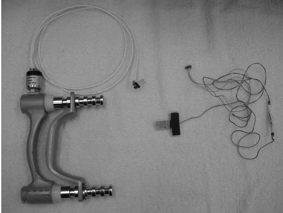
Figure 5.1. Instrumented gauges for grasp force measurements.
