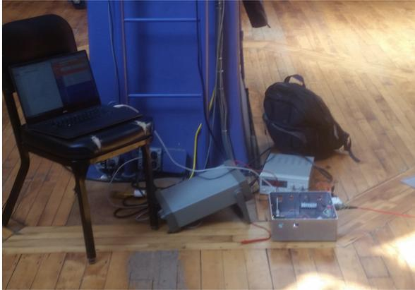
(a) The readout portion of the PSS testing and calibration setup. This picture shows the Lab-jack T7 box, power supplies, and a laptop to display signals read by the T7. The red cable on the right is connected to the purple one in Figure 2.4b.
