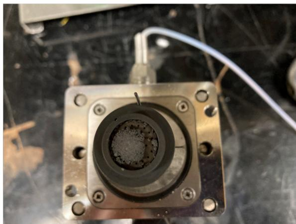
**Figure 5.5:** Images of the  $\text{MoO}_3$  precursor and A900 product of the in situ ammonolysis reaction show significant densification after the reaction.
