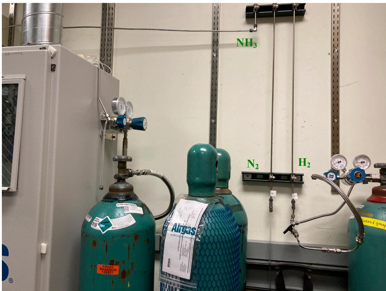
1. Put regulator on tank and connect tank to appropriate gas line.
