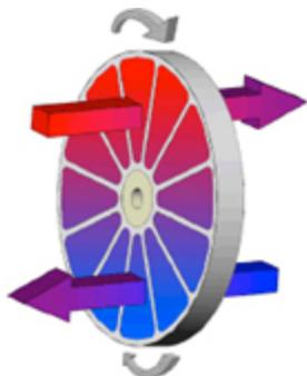
Figure 1: Turbo heat exchanger (process-heating.com)
