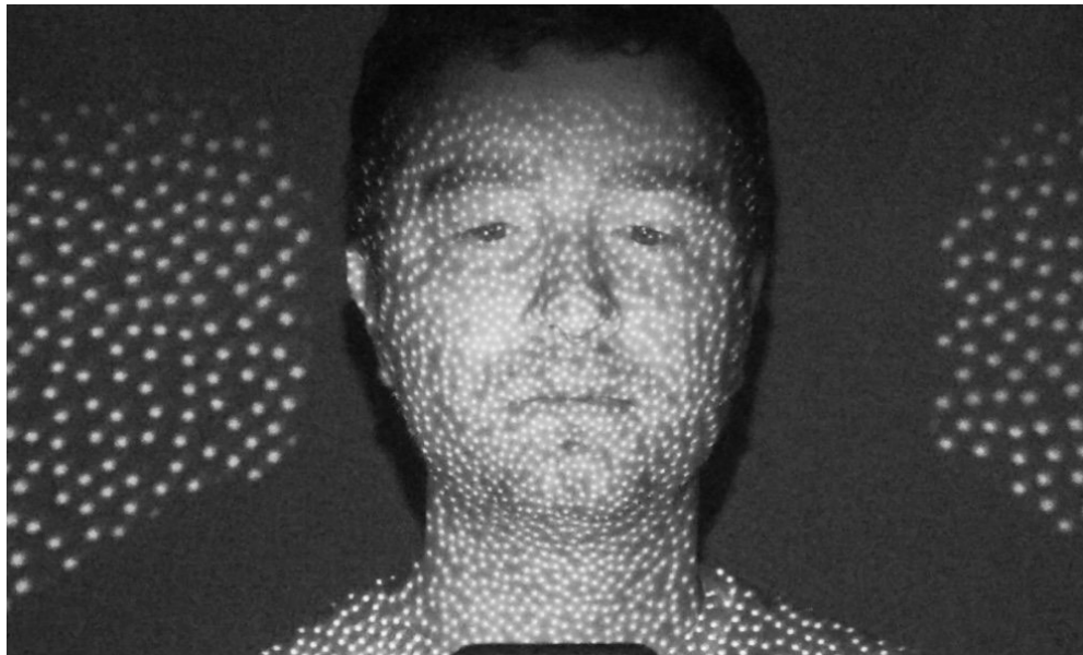
Figure 4-5. Image captured via infrared camera showing Apple's TrueDepth camera and facial recognition system in action. Image source from https://www.idropnews.com/news/app-developer-access-to-truedepth-camera-worries-privacy-advocates/57116/
