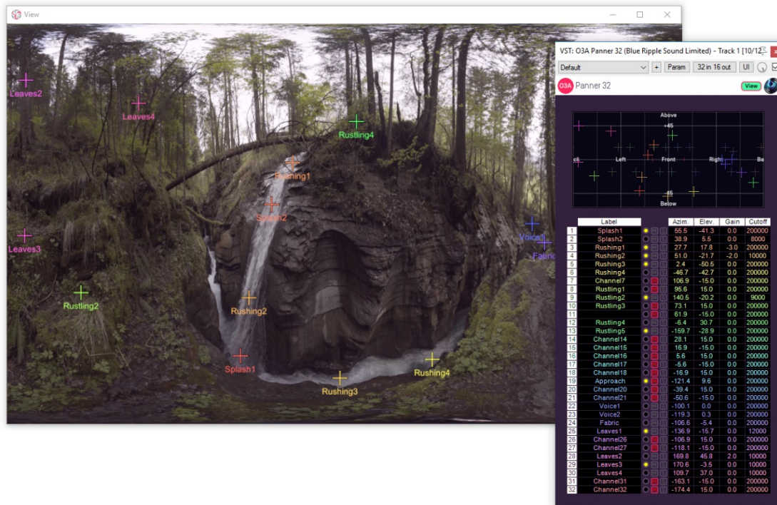
Figure 4-27. Screen capture of editing a spatial mix while viewing a 2D representation of a 360 video via Blue Ripple Sound’s O3A View app. Image source from: https://www.blueripplesound.com/products/o3a-view
