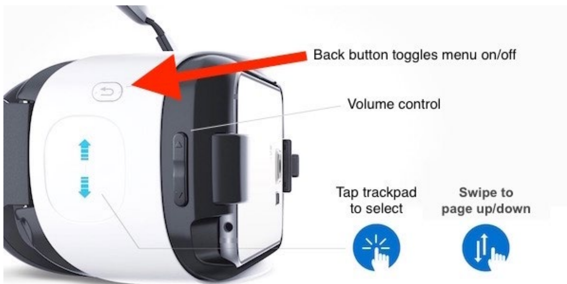
Figure 4-11. Image showing the Gear VR's simple onboard controls. Image sourced from https://groovr.zendesk.com/hc/en-us/articles/115002822988-Using-GrooVR-GearVR
