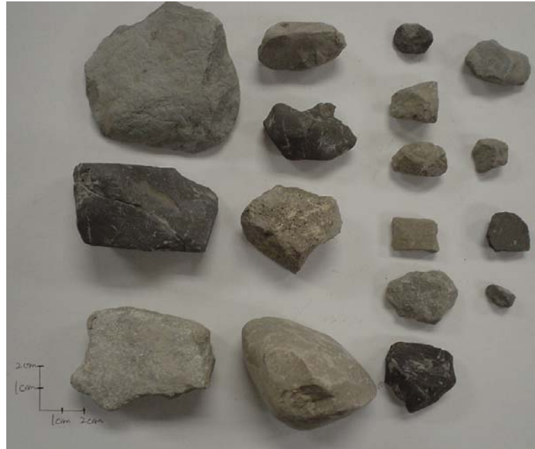
Figure 3-8 Selected shale and dolomite fragments from the block samples
