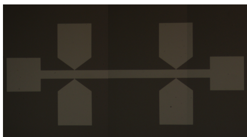
Figure 4.2: True color optical micrograph of the completed Hall bar with normal lighting. The 2DEG appears light due to the clear crystal background, but will appear dark to the naked eye.
