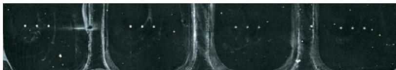
**Figure 9:** Photograph taken by the Verigene ID System of spotted glass slide following bio-bar code assay and scanometric and silver staining with the white spots, indicating the presence of bar-code DNA.
