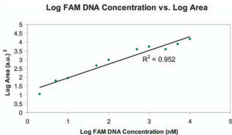
Figure 5: Standard curve for FAM-labeled DNA exhibiting the linear relationship between fluorescent DNA concentration and emission area.
