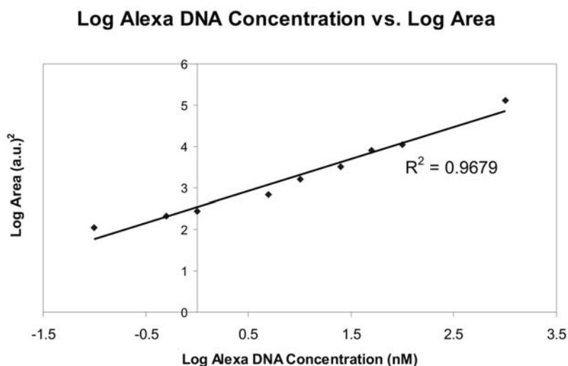
Figure 7: Preliminary results for standard Alexa-labeled DNA curve showing a linear relationship between Alexa-labeled DNA and emission area from picomolar to nanomolar range.
