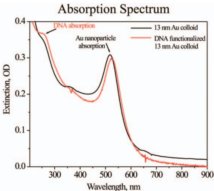
Figure 3: Absorption spectrum of 13 nm gold colloid compared with the absorption spectrum of DNA functionalized 13 nm gold colloid.
