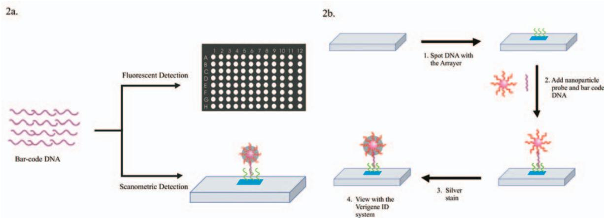
Figure 2: The two methods of DNA detection used are shown here with the scanometric schematic as developed by the Mirkin lab.
