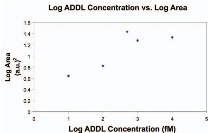
Figure 6: Increasing fluorescent trend for the FAM-labeled bar-code DNA collected from the bio-bar code assay for ADDL detection.
