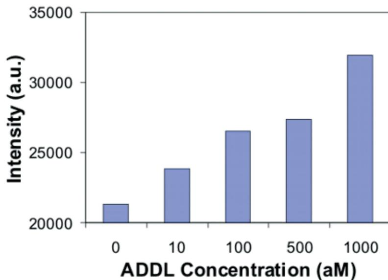
**Figure 10:** Increasing trend of spot intensity with increasing ADDL concentrations shown here indicates the ultrasensitivity of the scanometric method. The assay has a dynamic range between 0–1000 aM.
