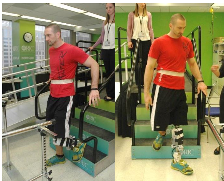
Figure 4.2: A transfemoral amputee wearing the powered knee-ankle prosthesis demonstrating various transitions from stair descent to level-ground walking.
