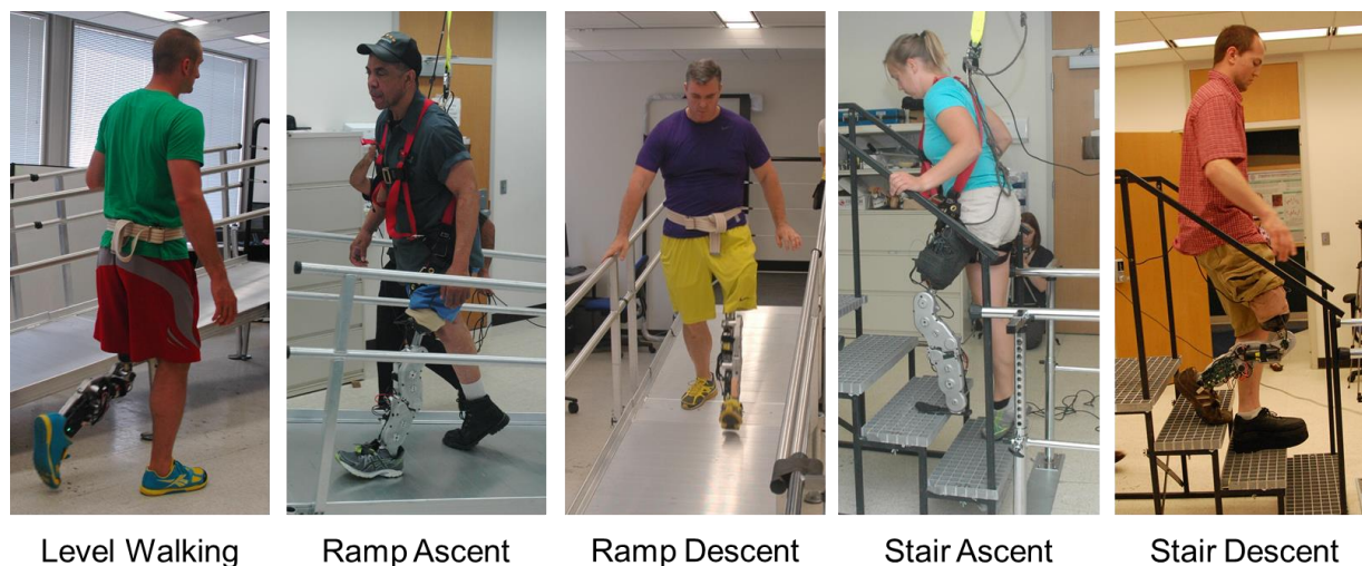
Figure 3.2: Photographs of amputee subjects completing the locomotion circuits with the programmed locomotion modes. The figure shows examples of the different modes of the powered lower limb prosthesis. The prosthesis transitioned between these modes as the amputee subjects completed the locomotion circuits.
