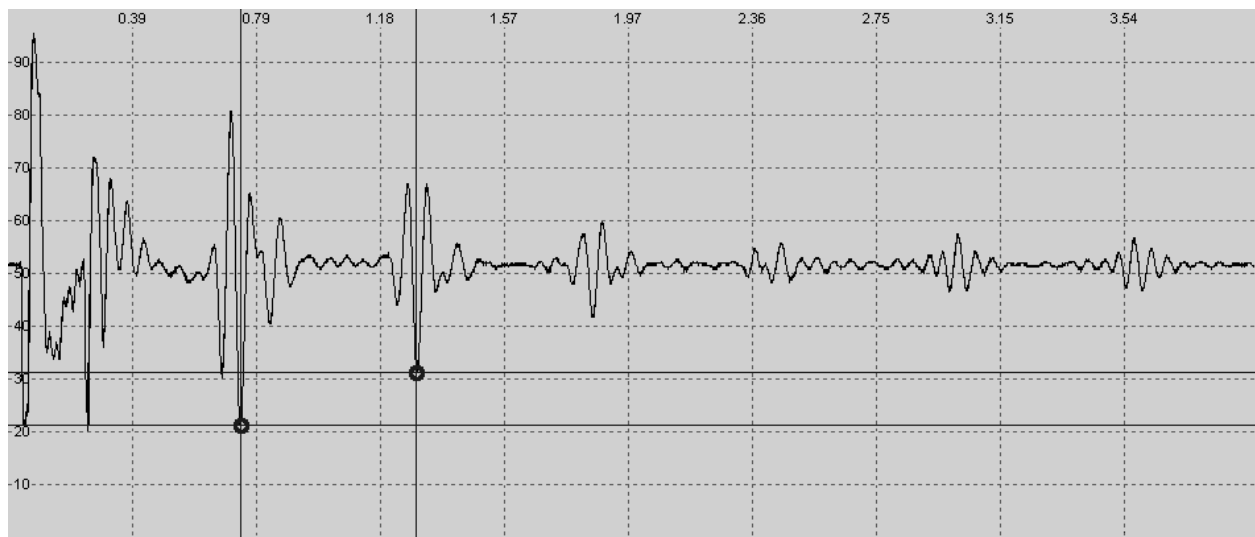
Figure 4.7. Digital readout from the ultrasonic inspection system of wave amplitude versus time.
