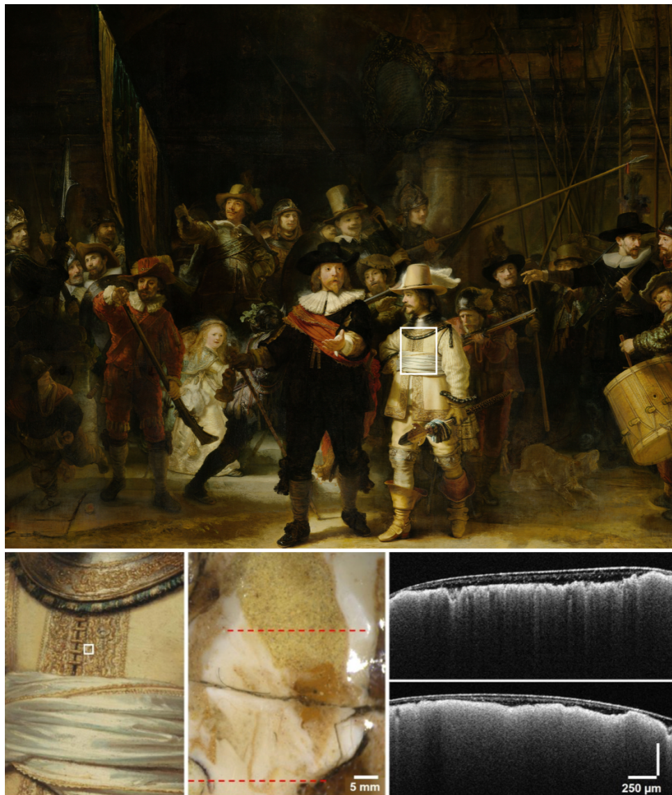
Figure 2.4. A 2D virtual cross section (B-scan) done in a small region of the shirt of Willem van Ruytenburch [27]. The varnish layers are clearly visible as well as the surface topography of the paint layers.
