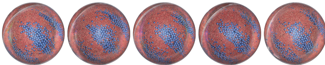
Figure F.2. Five segregation experiments in a half-full spherical tumbler after 30 iterations of protocol (57^\circ, 57^\circ, 90^\circ) rotated at 2.6 rpm for particle size ratio R = 3.56 and f = 15\% . Segregation pattern for (57^\circ, 57^\circ, 90^\circ) is repeatable.
