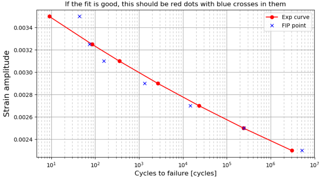
Figure 3.8. FIP predictions versus statistical model of fatigue life, used for calibrating the FIP parameters. The FIP points shown minimize the cost function in Eq. (3.15). A perfect fit would overlay the blue crosses and red dots. Because this FIP is designed for HCF, it seems reasonable that for lower number of cycles the fit is mismatched (i.e. low-cycle mechanisms are not captured)
