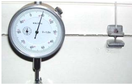
Figure 3-9: Large displacement of joint between two pieces of molding verified as dial gauge, a) the 6/18/04 and b) the 7/28/04.
