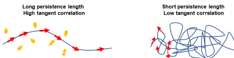
Figure 1.10. Schematic of persistence length of fibers. Long persistence length (left) in a thermal environment corresponds to higher bending stiffness, and higher correlation of tangent vectors. Short persistence length (right) corresponds to lower bending stiffness, and shorter correlation of tangent vectors.
