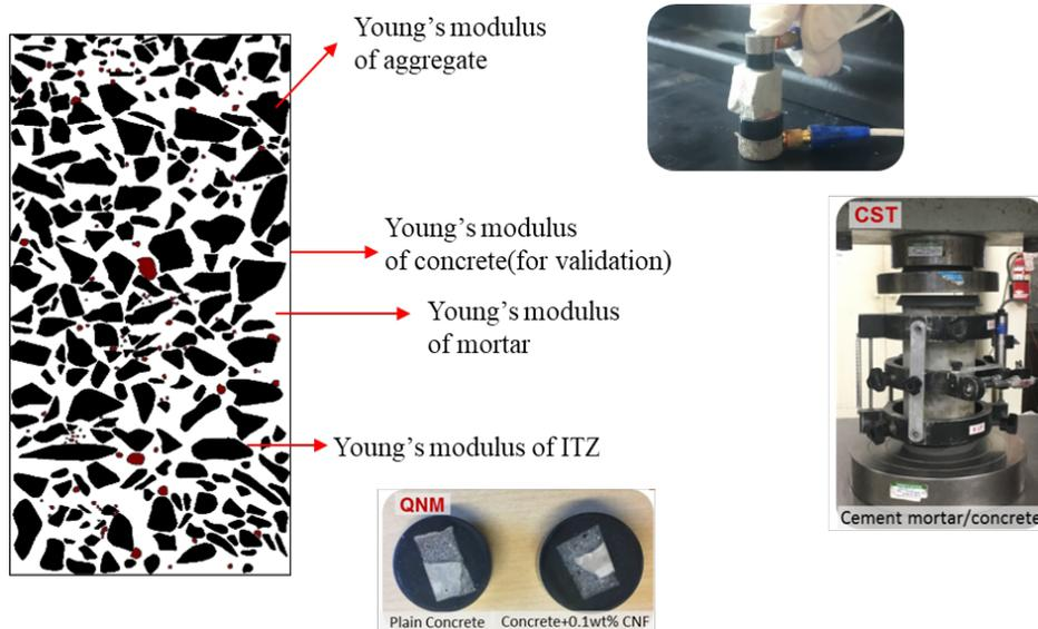
Figure 5.5 Input parameters for the simulation model
