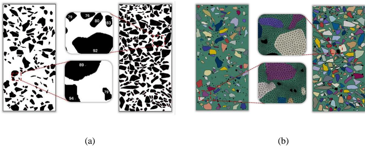
Figure 5.6 Aggregate profile in FEM model
