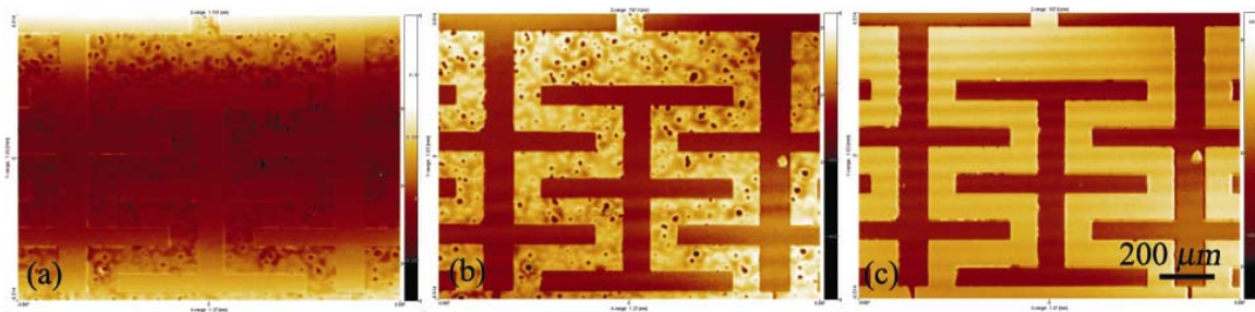
Figure 2-19: BDL pattern transfer by etching metal: Optical profile images of (a) after the PDMS is patterned (b) after the Cr layer is etched, and (c) after removing the PDMS by light mechanical polishing.
